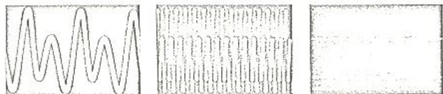
Fig. 1 The same artificially generated waves having a strong second harmonic, photographed at three different sweep speeds to show the origin of oscillograph patterns such as those seen in figures 6 and 7. Note how the peaks and inflections form bright spots (owing to the lower velocity of the cathode ray trace), and how at the slowest sweep speed (shown on the right) these spots fuse into continuous lines.
